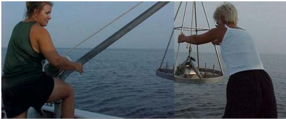
Figure 1. Young grab sampler used to collect sediment and benthic samples.
