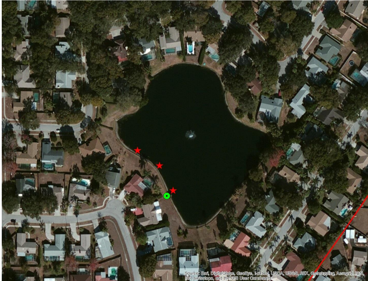
Figure 16. P202 stormwater sampling location using an autosampler (green circle) and stormwater pond surface sampling locations (red stars).
